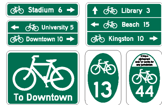
Directional signs (top), regional route signs (bottom right), and confirmation signs (bottom left).
