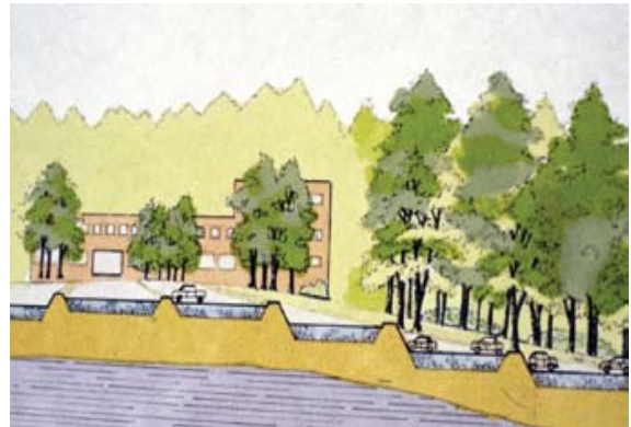
Figure 3 Slope stepping with berms Source: Andropogon
